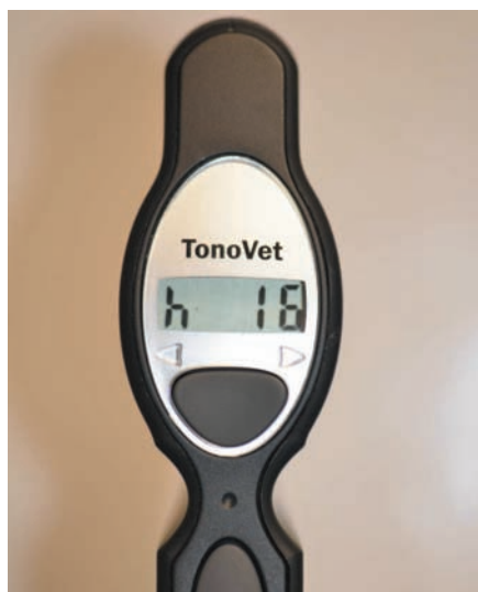
Figure 2: The display screen for the TonoVet. The letter h on the left of the screen indicates the horse setting.
